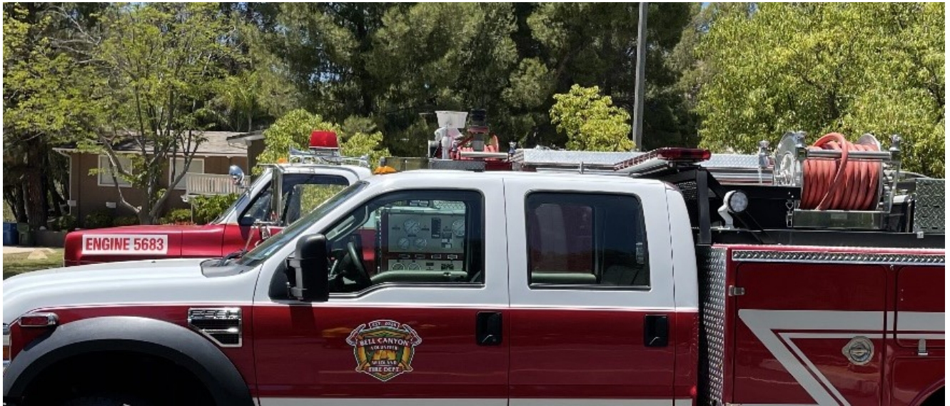
Brush 1 is a Ford F-550 4x4 with a 280 gallon tank.
