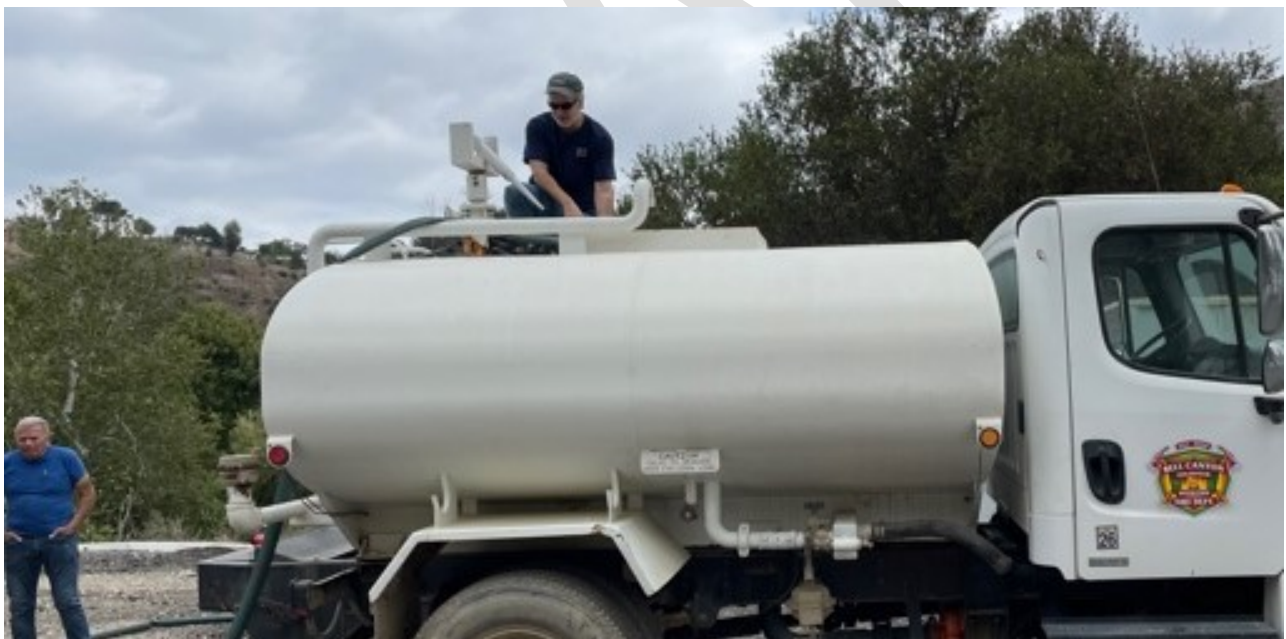
BCVWFD's Water Tender has a capacity of 2,000 gallons and will primarily be used to refill fire and brush trucks.
