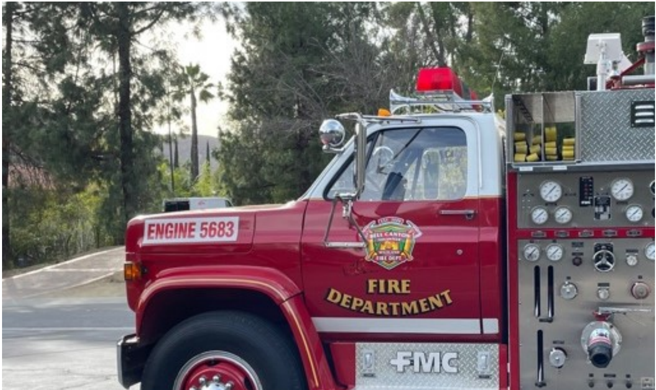
Engine #83 is a Type 2 FMC engine with a 500 gallon tank and is the department workhorse.
