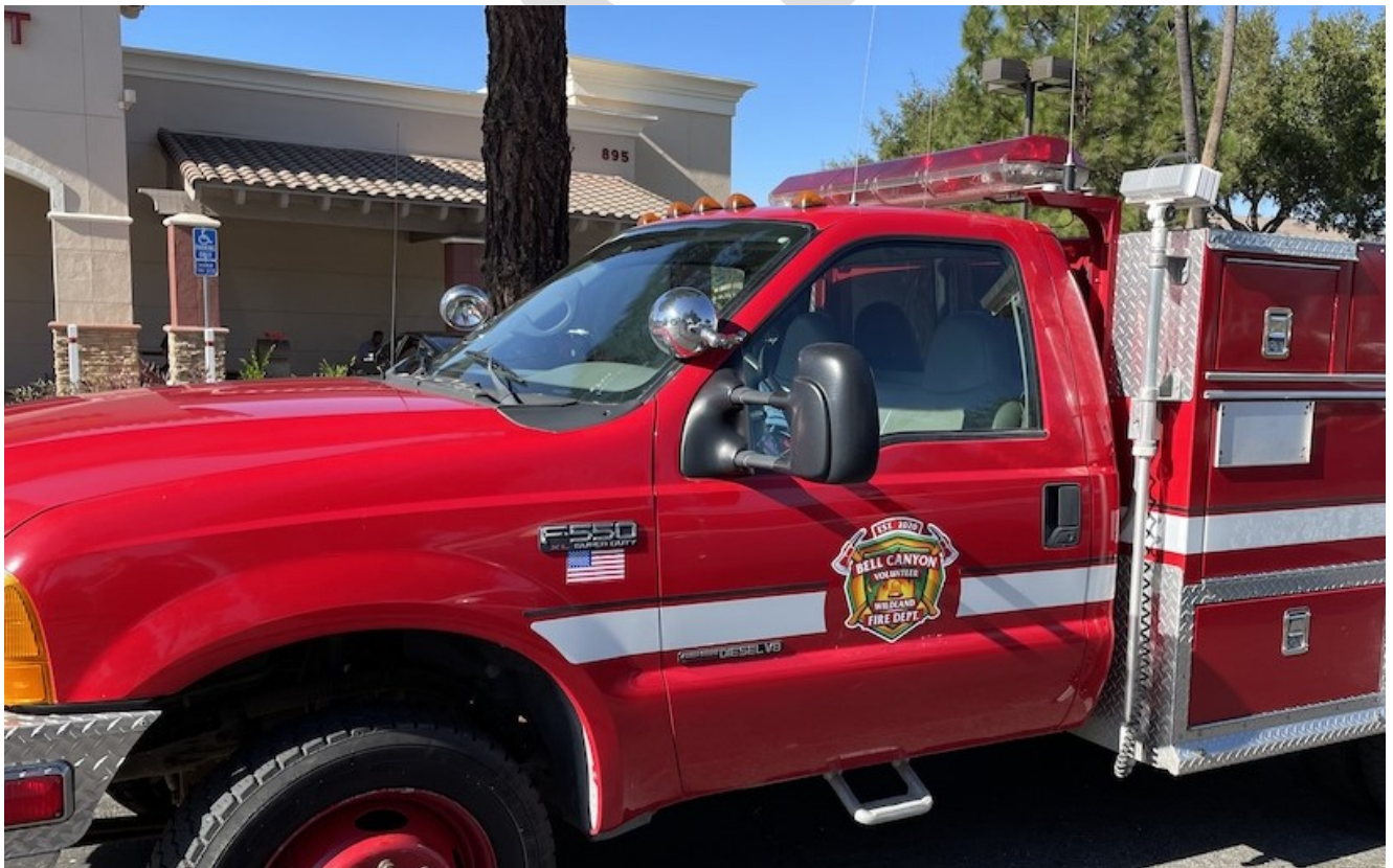
Brush 2 is a rapid response Ford F-550 4x4 with a 300 gallon tank.
